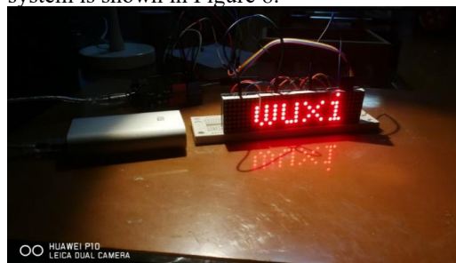
Figure 8 The physical object of the LED dot matrix display system
